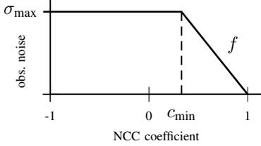
Fig. 3. Linear mapping of correlation measure to the Kalman filter's observation noise.
