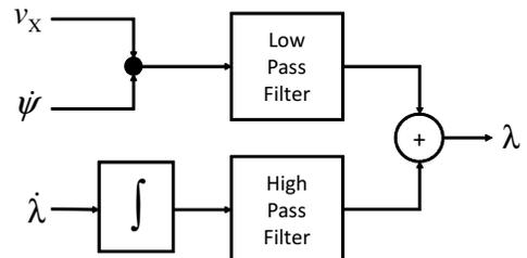
Fig. 4. Basic Principle of Combined Filter Method
