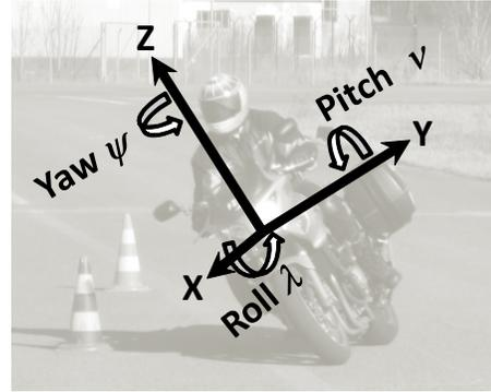
Fig. 1. Illustration of the motorcycle coordinate system.
