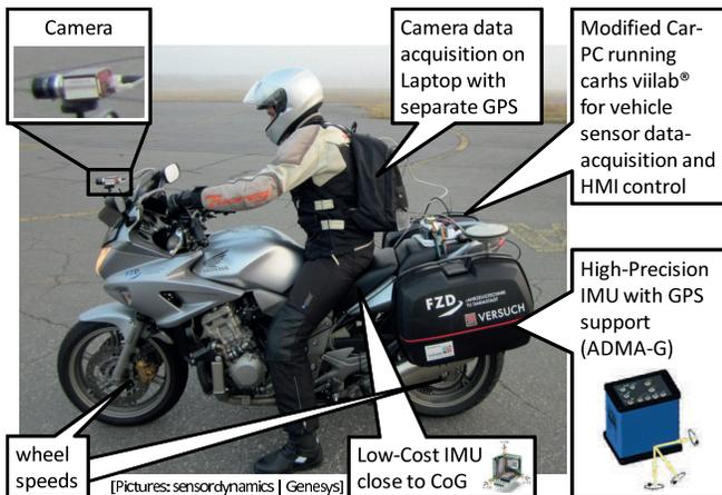
Fig. 5. Setup of test motorcycle
