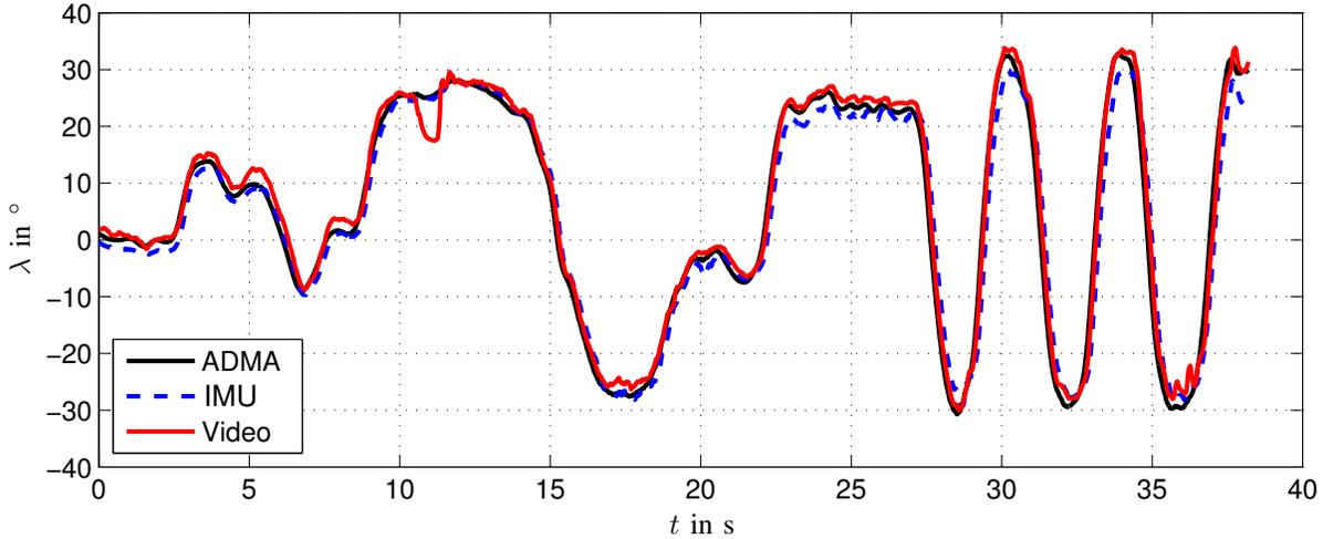
Fig. 7. Reference values (ADMA) and estimates of the roll angle for the IMU-based Kalman filter method (IMU) and the Video-based method (Video)
