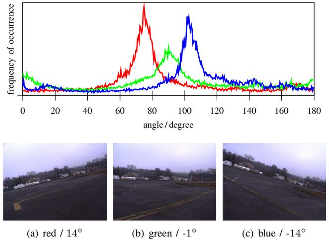
Fig. 2. Normalised orientation histograms of three closely recorded images and their corresponding ground truth roll angle.
