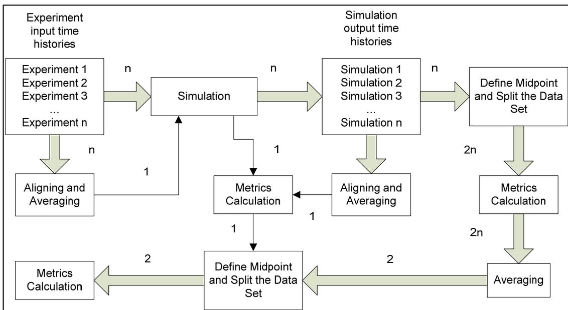
Figure 4.27 Summary of simulation data handling methods
