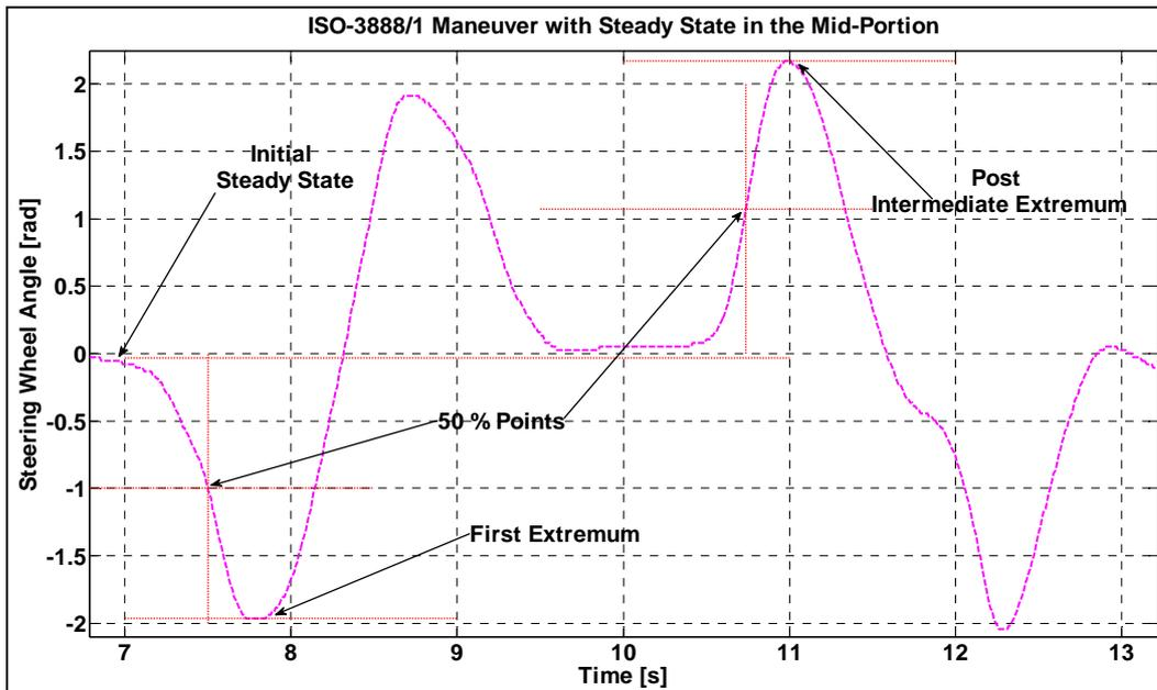
Figure 4.24 Definition of reference points according to (a)
