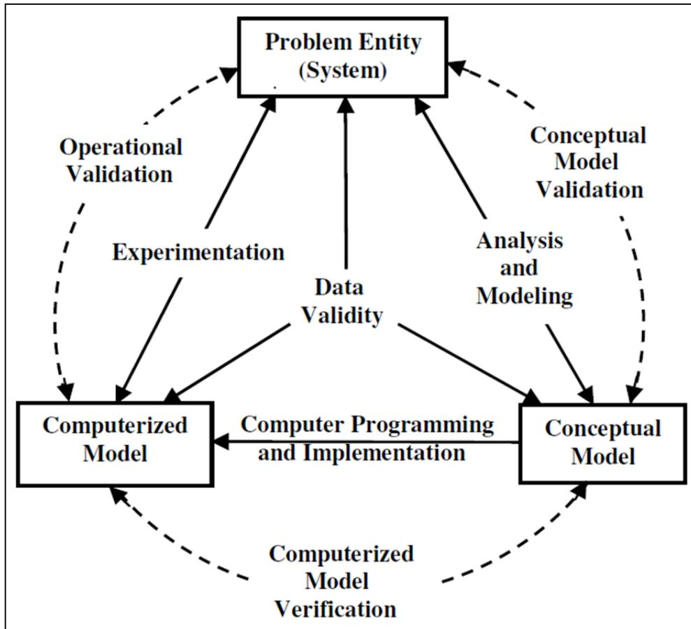
Figure 2.1 Simplified version of the modeling process<sup>34</sup>
