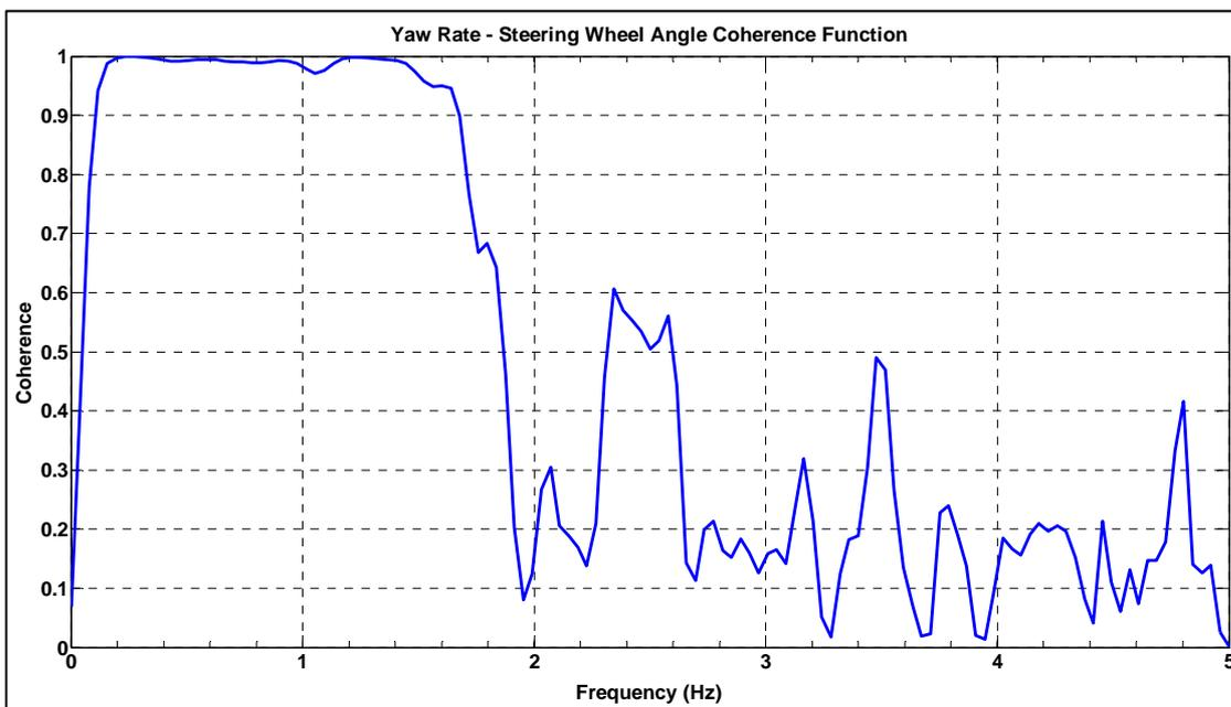
Figure 4.14 Sample Coherence Function of the Yaw Rate
