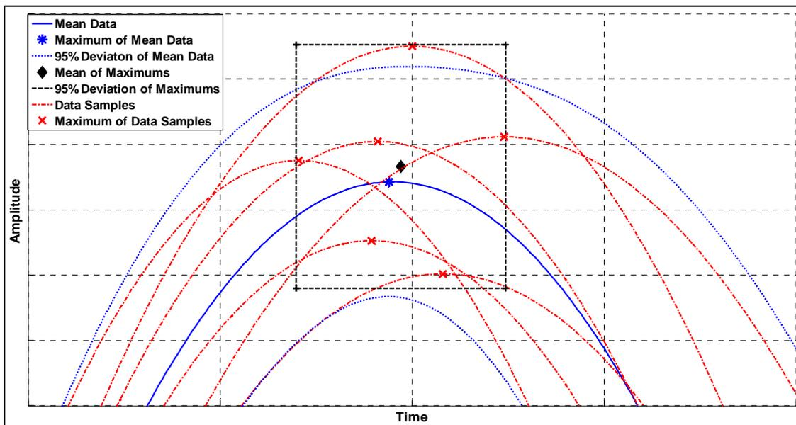
Figure 4.7 Graphical Explanation of MVW Concept: The extremum (and the deviations) obtained by averaging the signals, is not equal to the average (and the deviation) of the extrema of the signals.
