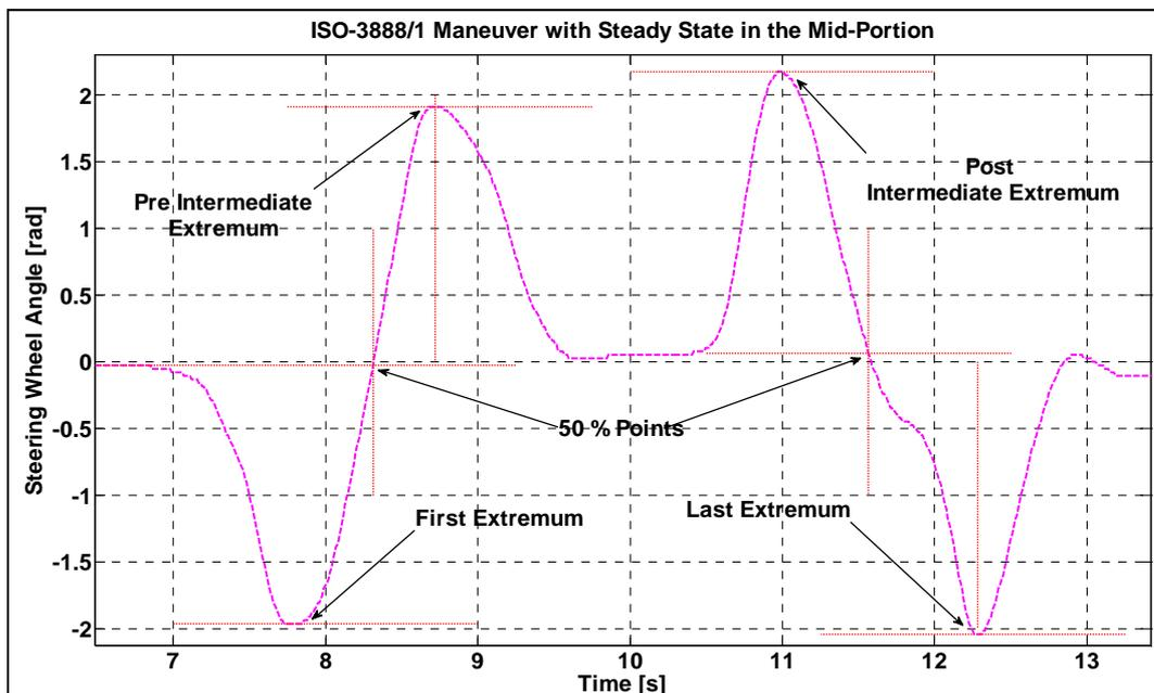
Figure 4.25 Definition of reference points according to (b)
