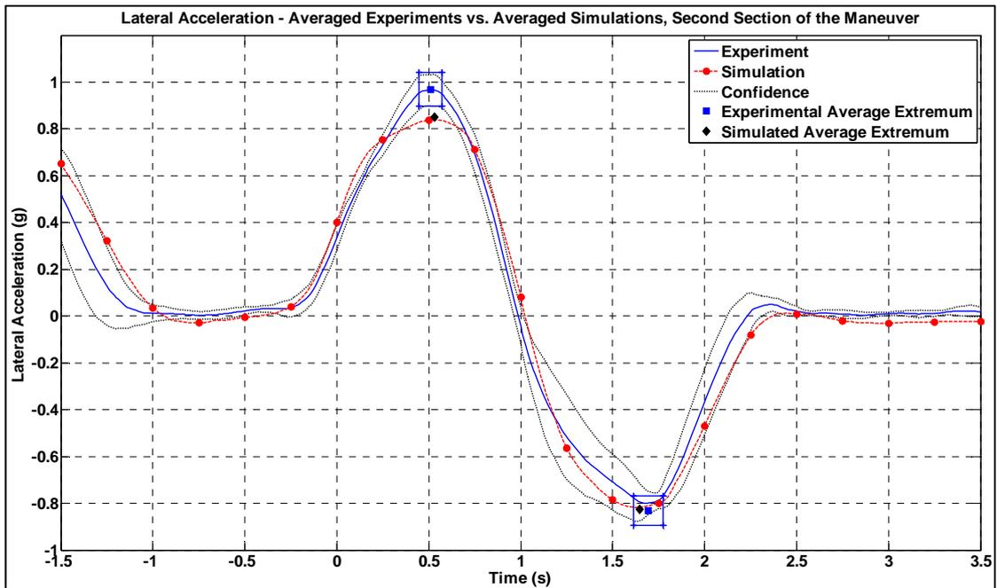
Figure 4.34 Lateral Acceleration EDZ vs. Averaged Simulation – The Second Move
