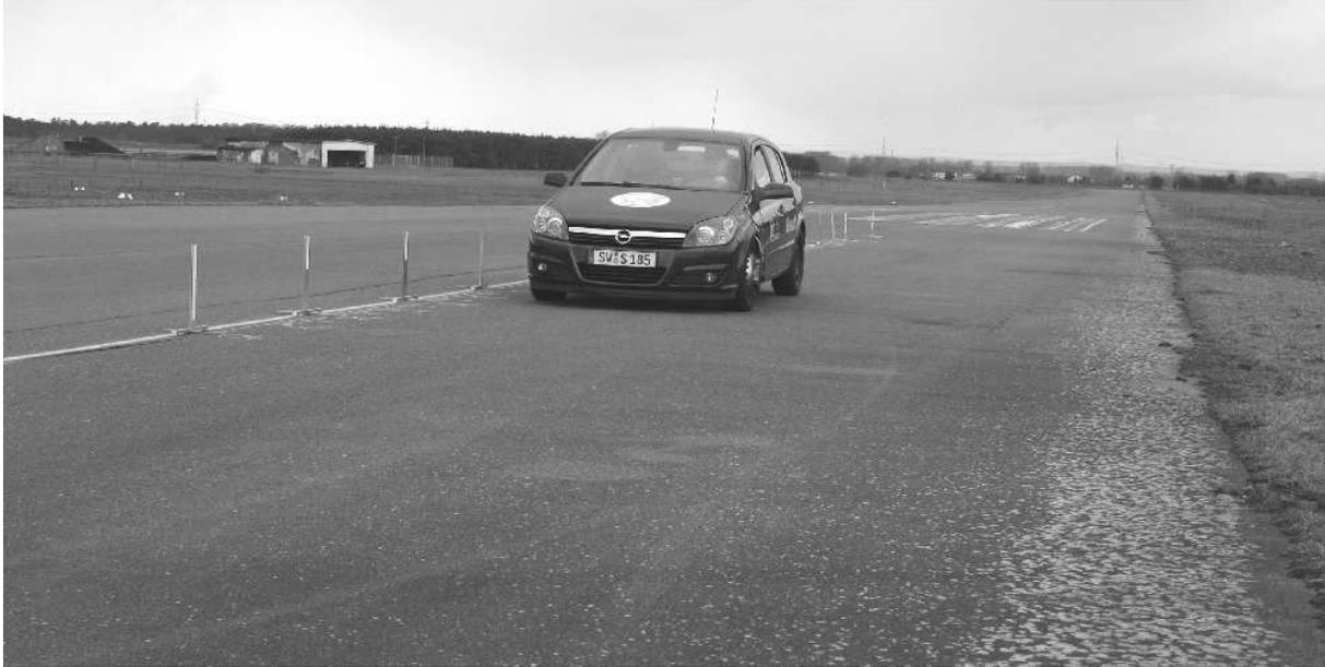
**Figure 3.15:** Test track ‘Standard Road’ (an airfield) on which part of the braking tests are executed with the testing vehicle during a braking procedure.
