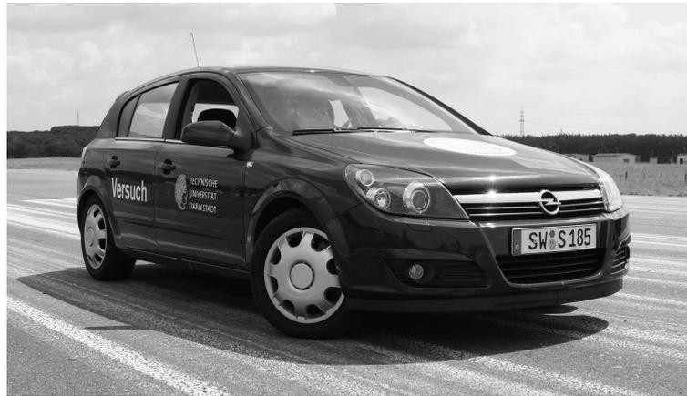
**Figure 3.3:** The testing vehicle which is used for all experimental testings Opel Astra H 2.0i 16v Turbo on the testing track ‘Standard Road’.
