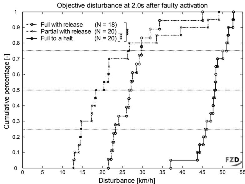
Figure 5: Cumulated percentage of the disturbance (passenger car)
